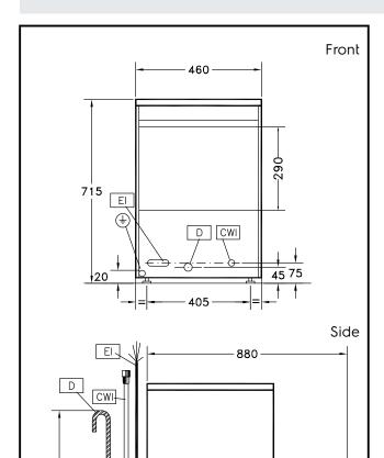
= Cold Water inlet 1 (cleaning) CWII Drain
